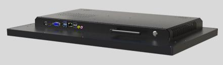
General Touch's breed of Closed Frame Touch computer is characterized by its unified design with AL Alloy frame edges. This sleek and sturdy contraption is loaded with enticing features and options that cater to different requirements including operating on Android, Windows and Linux platforms. The Android version is equipped with a Rockchip processor, while the Windows and Linux versions utilize powerful Intel processors.
